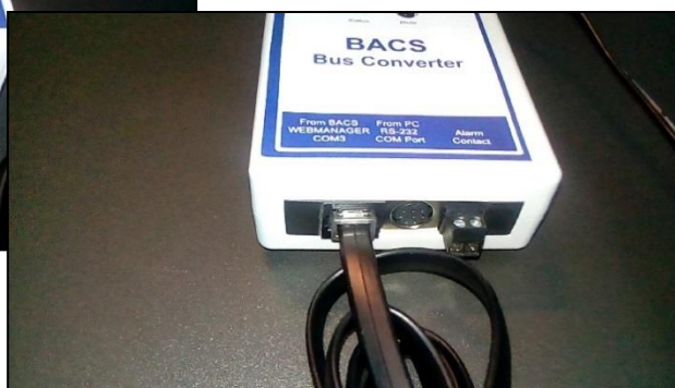
... to the COM 3 port of the BACS-Bus Converter
